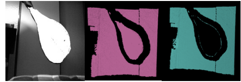
Fig. 3: Point cloud of waving tennis racket segmentation(each picture represents: image after segmentation, original point cloud, point cloud after segmentation)
