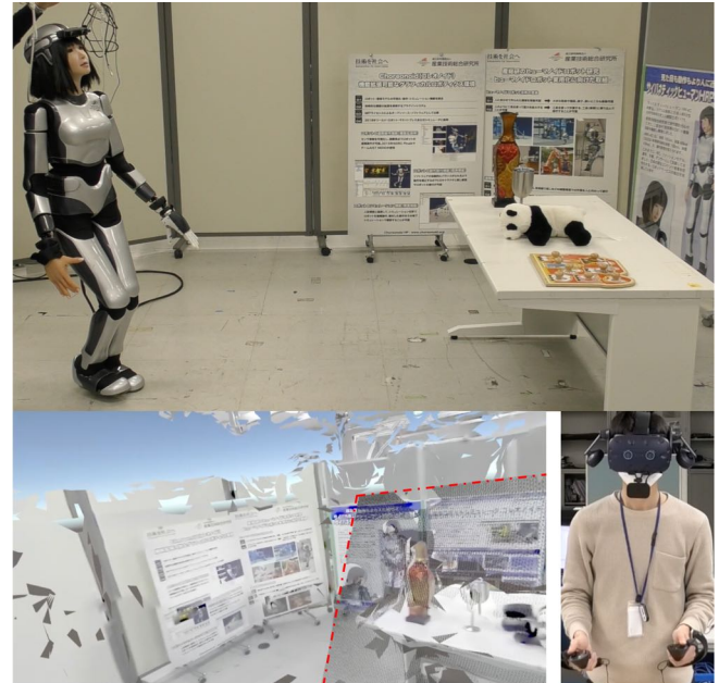
Fig. 1. Proposed tele-visualization. Top side: real scene, left-down side: virtual scene, the real-time point cloud is shown in the area inside the red dot line, the area outside denotes the constructed mesh, right-down side: operator.
