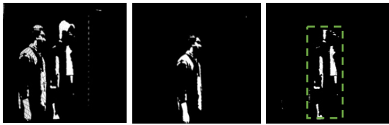
Figure 8. Dynamic binary pixels separation(from left to right: (a)DiffImg, (b)Dyna_LastImg, (c)Dyna_CurrentImg)
