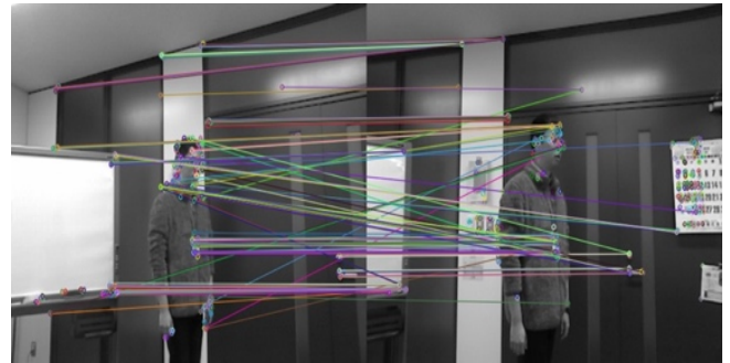
Figure 1. Example of incorrect keypoint matching result in a dynamic environment
