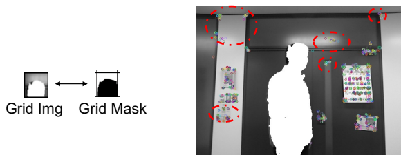
Fig.13 Split the image and mask into 30*30 patch
