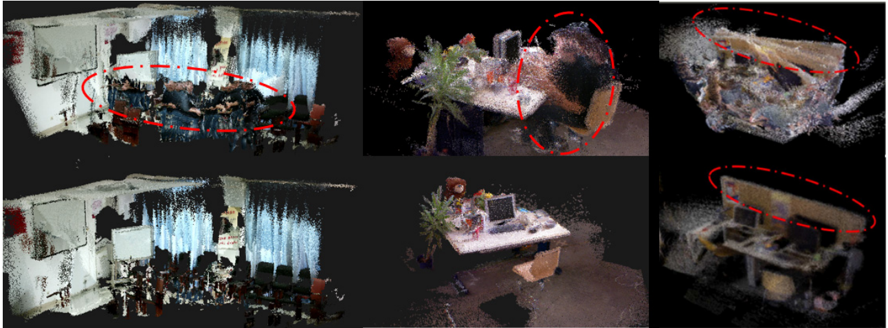
Fig. 18. Comparisons between the dense RGB point cloud maps. The top row shows the RGB-D images directly projected by the original ORB-SLAM2 estimated pose, while the bottom row shows the result of our proposed framework.
