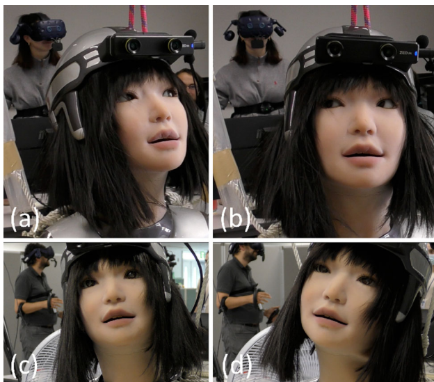
Fig. 22 Neck motion: looking left-right using the yaw joint in a and b , and head tilting using the roll joint in c and d
