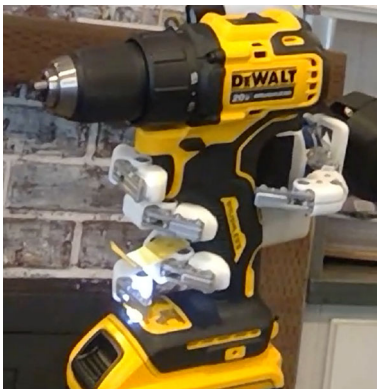
Fig. 13 Power grasping (heavy wrap while operating drill)
