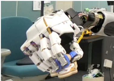
Fig. 12 Precision grasping (tripod grasping of a puzzle piece by its knob)
